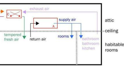
A: Air Handler B: Heat Pump C: Energy Recover Ventilator
