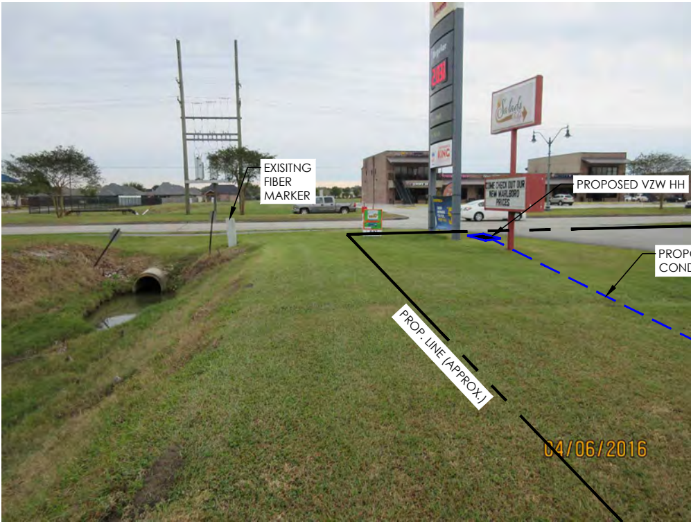
PROPOSED HANDHOLE LOCATION & CONDUIT ROUTE NOT TO SCALE
